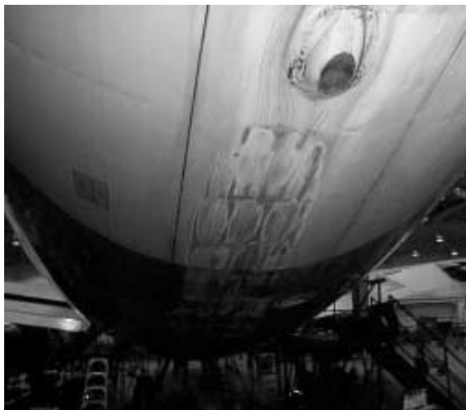
A300 tailstrike damage
