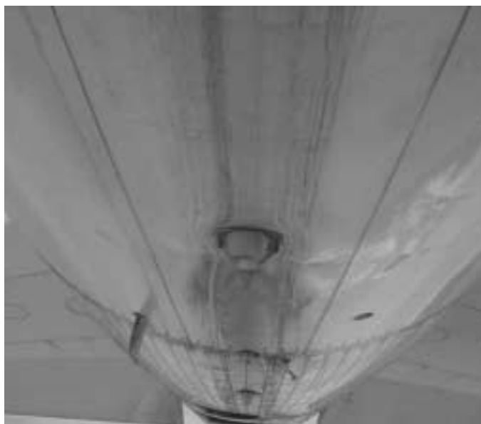
A300 tailstrike damage
